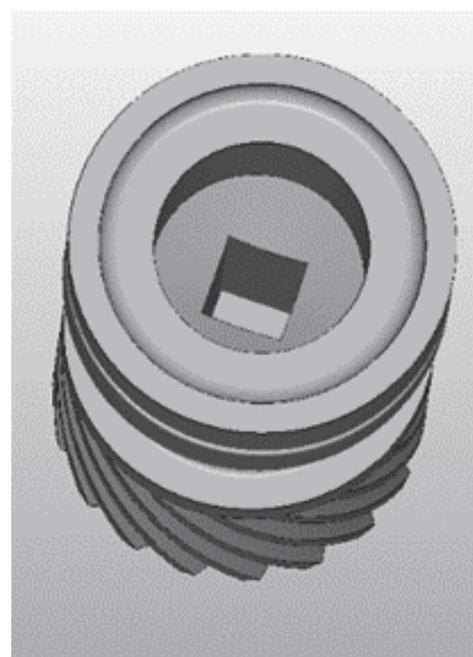
Fig.3. Component that is not producible via chip machining methods
