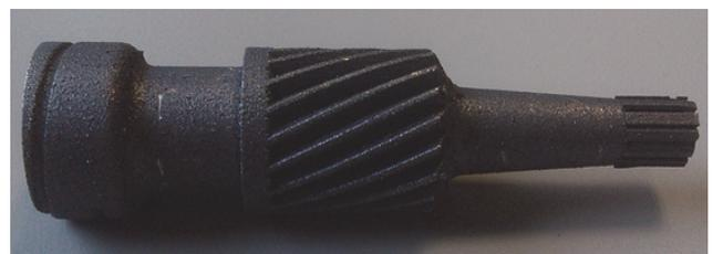
Fig.5. Part without surface finishing
