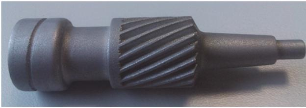
*Fig.6. Sandblasting surface finishing*
